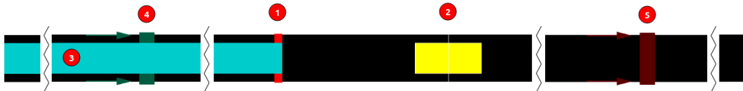
Figure 5.2: The simulation setup that was used for the model comparison. The horizontal axis has been truncated at the indicated locations for visibility reasons. Right after the traffic light at (2) is an E1 induction loop detector (2), visualized as a yellow rectangle, which is used to count the number of departures within a loop (used by the departure-counter tool). The long turquoise rectangle (3) represents an E2 lane area detector, which can measure the actual queue length, and spans from the beginning of the lane to the traffic light. The entry (4) and exit (5) detectors of the E3 detector are used to measure delay and are located at 400m and 700m, respectively.
