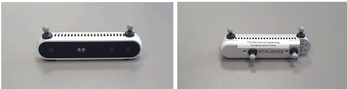
Figure 3.4: Intel RealSense D415 camera, which is used to obtain RGB videos of tumbling boxes.
