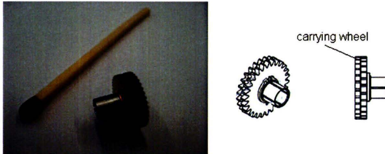
Figure 4.10: anti backlash gearwheel
