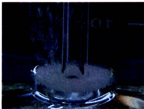
Figure 19: Close-up of the diffuser used in the water bath
