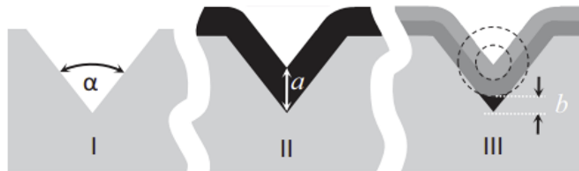
Figure A.4: Schematic overview of corner lithography [106].
