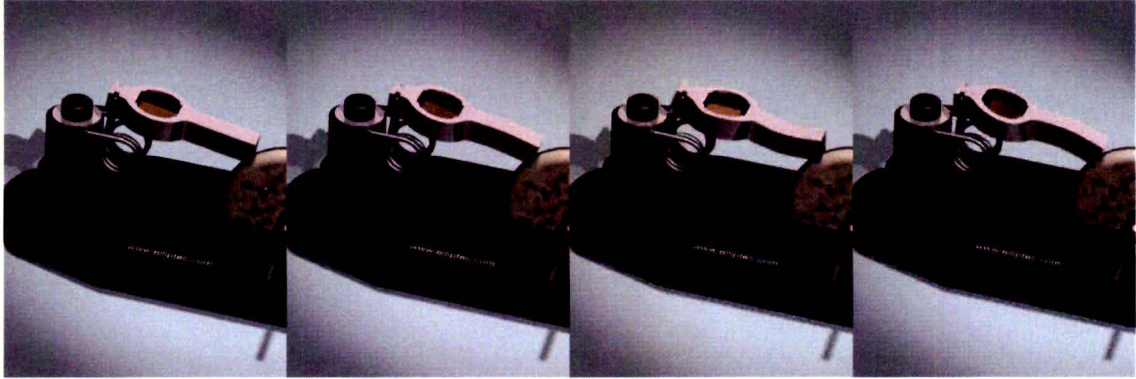
Figure 2.3: Vibration mode of Elliptec motor as shown on: www.elliptec.com .
