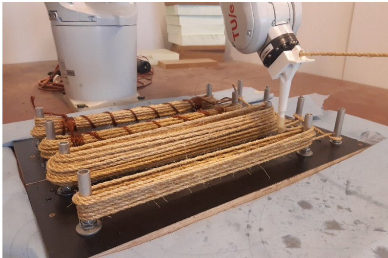
Figure 65: Photograph of initial winding session
