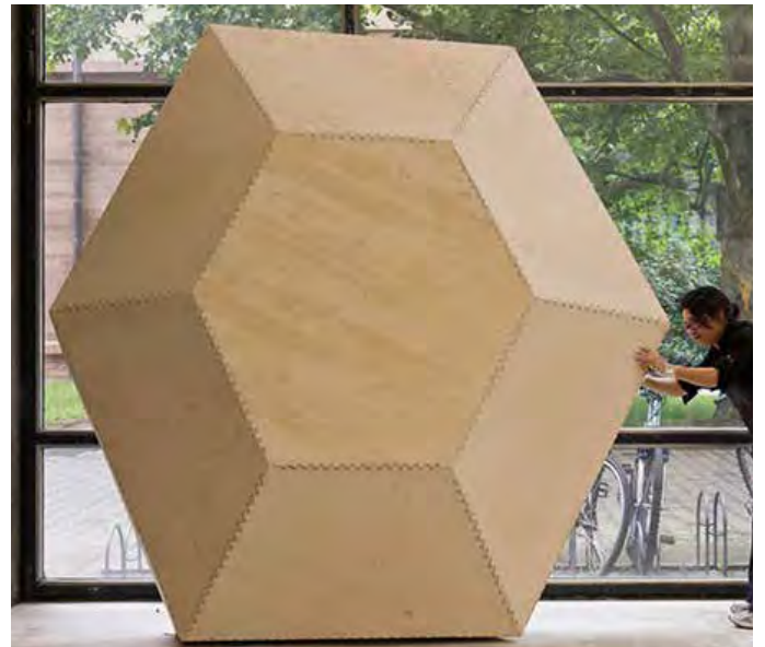
Figure 22 (ICD / ITKE University of Stuttgart, Roland Halbe, 2011) Assembled plate cell, ready to go to the site.
