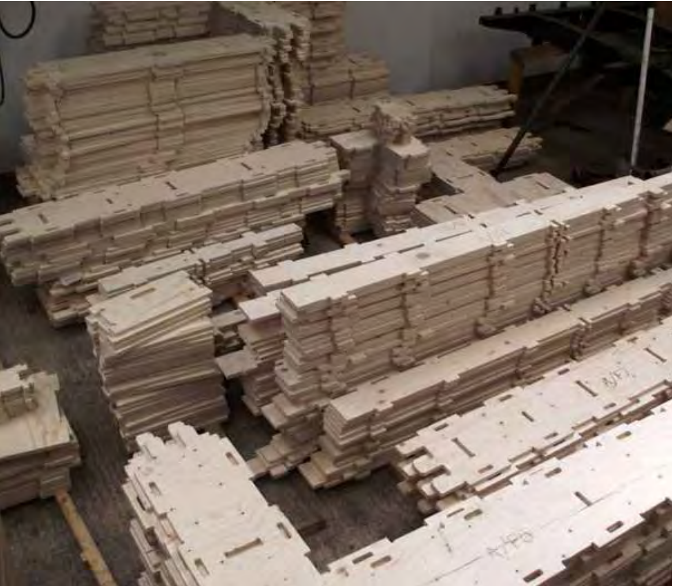
Image 47. Parts of a Wikihouse (urbanNext,2020)
