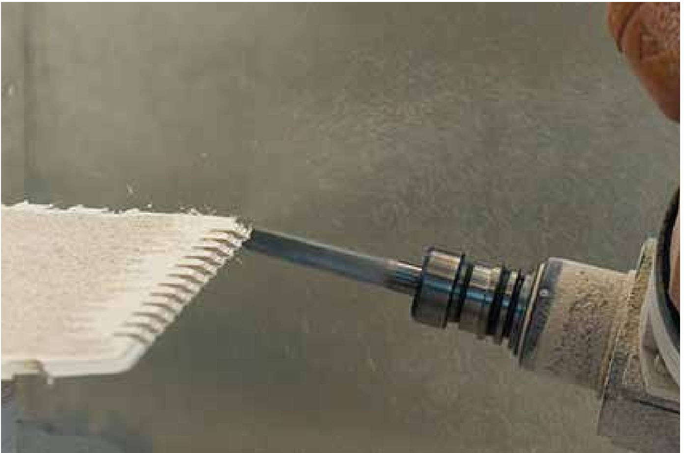
Figure 18 (ICD / ITKE University of Stuttgart, Roland Halbe,2011) Milling of joinery edges.
