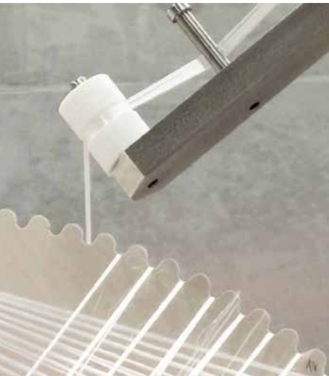
Figure 40 (ICD/ITKE University of Stuttgart, 2012) The fibers are wound by the 6-axis robot on a temporary framework placed on a turntable, creating a 7th axis.
