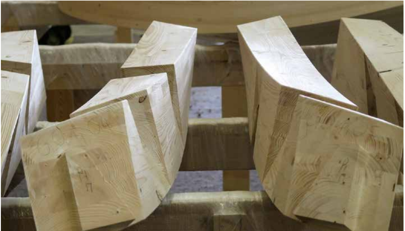
27. Timber element after processing with CNC milling (Marks Barfield Architects, 2020)
