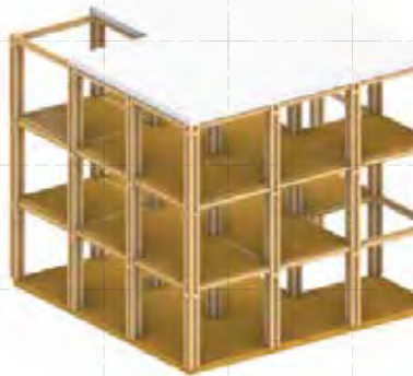
Floor & roof plates
