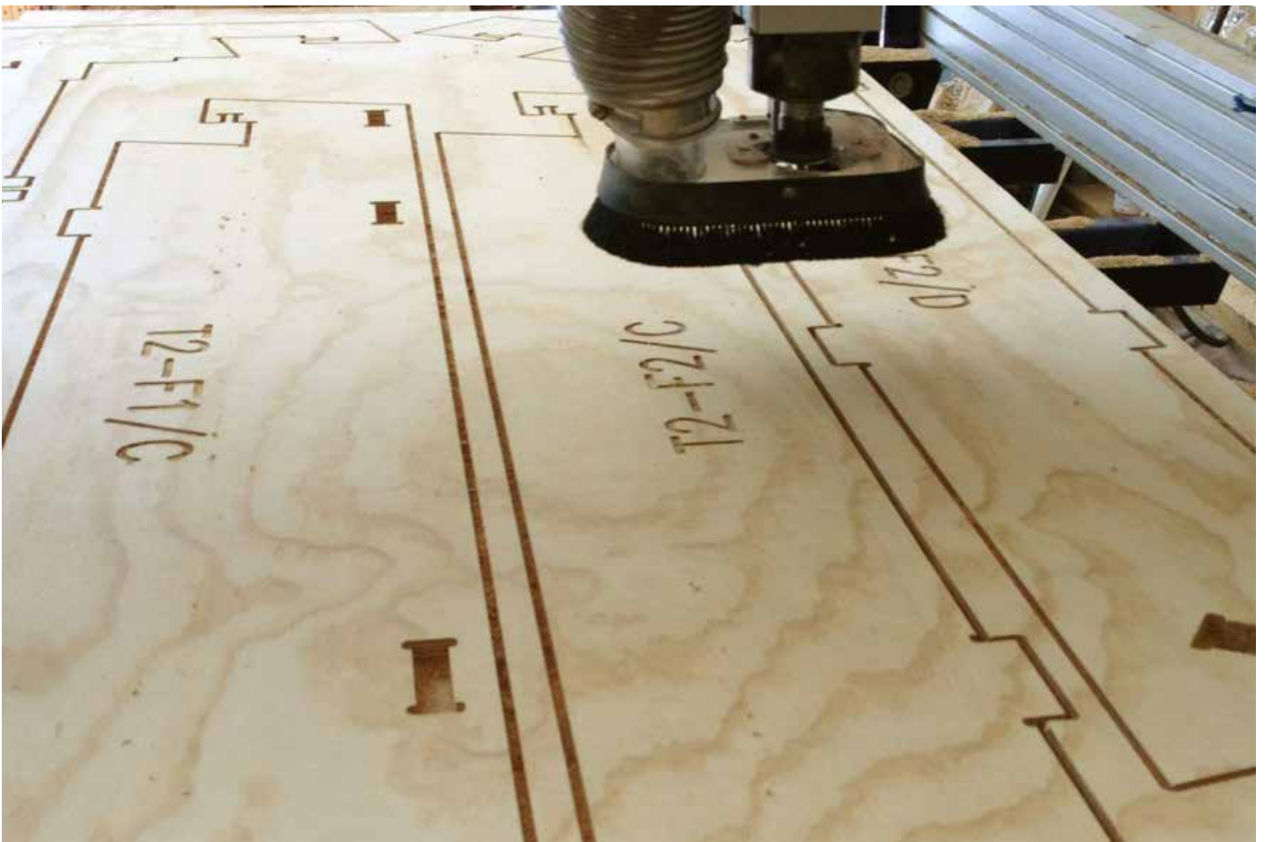
2. CNC routing (Open Systems Lab,2019)
