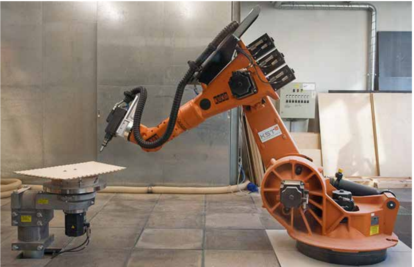
Figure 19 (ICD / ITKE University of Stuttgart, Roland Halbe,2011) Off-site fabrication process using CNC milling for the plate cells.
