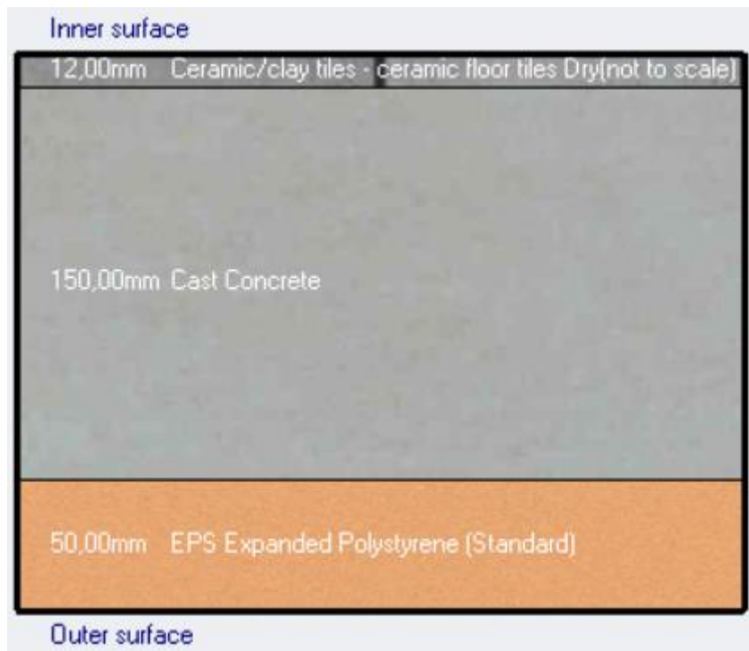
Figure 46: Detail of the ground floor of the freestanding house in DesignBuilder (low insulation)
