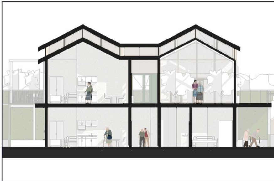
Figure 9.44: Section of the assisted living unit
