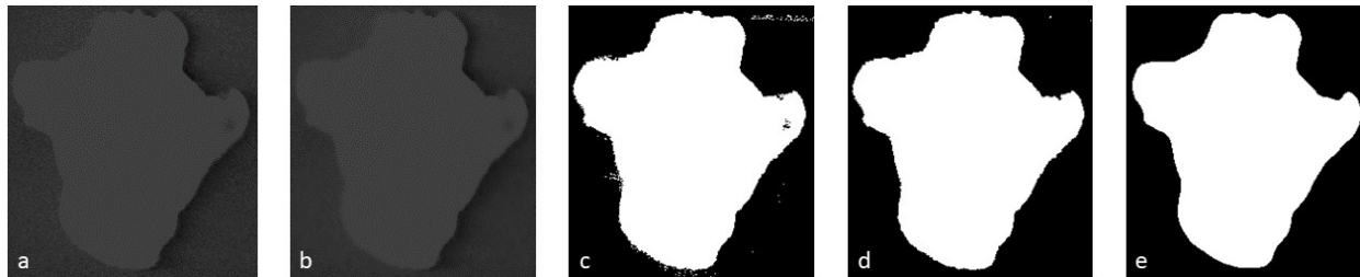
Figure 15: Example of image segmentation: a) Initial image. b) Smoothed initial image. c) Binarized image. d) Binarized image adapted to previous image segmentation method. e) Final image mask
