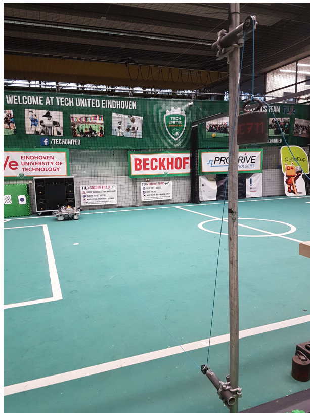
Fig. 17: Setup of experiments with a hanging mass connected to the platform with a rope via pulleys.
