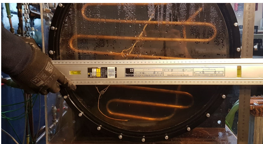
Figure 4.5: A typical measurement of the water height: The underside of the spirit level needs to align with the water level, the spirit level also needs to be level, which is indicated by the bubble near the hand. The height is measured at the intersection between the ruler and the underside of the spirit level.
