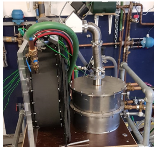
Figure A.3: Picture of the new condenser connected to the setup
