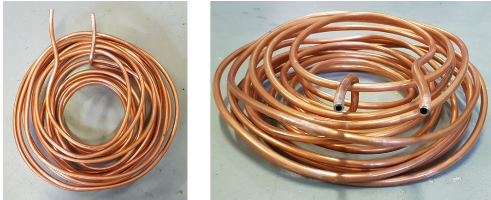
Figure 5.10: Left: a top view of the spiral heat exchanger. Right: a side view of the spiral heat exchanger.
