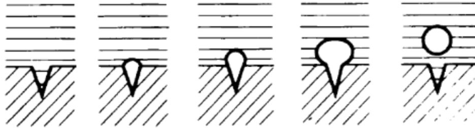
Figure 3.6: Visualization of bubble formation at nucleation site [27]
