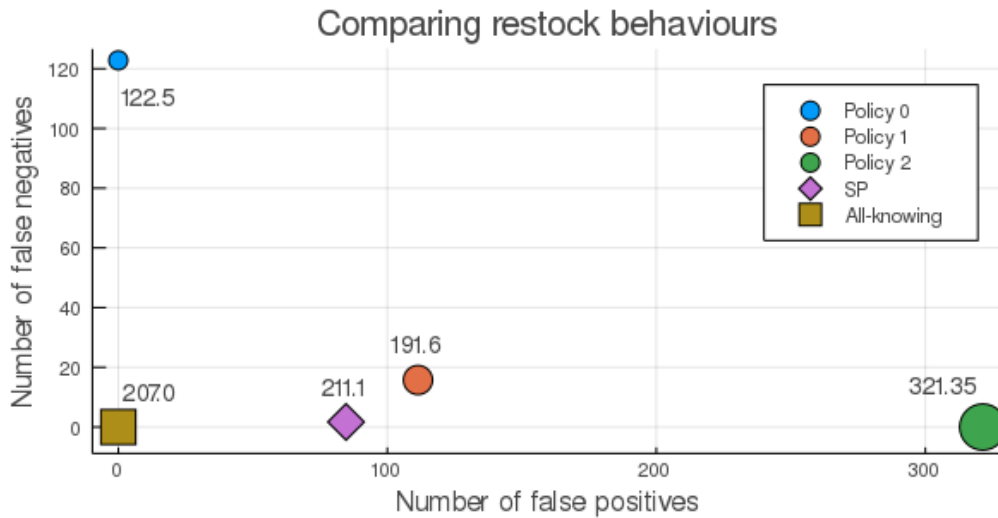
Figure 6.4: A comparison of the number of false positives and negatives for different deciders. The size and annotation of each marker indicates the total (average) number of restocks performed; note that a larger node indicates more restocks.
