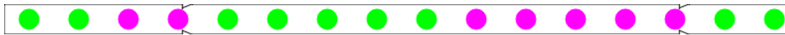
Figure 5.5: One end of a small corridor in which robots cannot move alongside each other. A few small windows are introduced in the workspace polygon. In this case, these windows are just too small for a robot to move through (e.g. 1.8 units wide). Another case would contain windows which are just big enough for robots to move through (e.g. 2.2 units wide). Note that since robots cannot move alongside each other, there is only one way to solve this setting, independent of the size of the windows.
