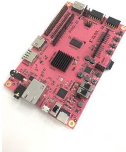
Figure A.2: The PYNQ-Z2 board
