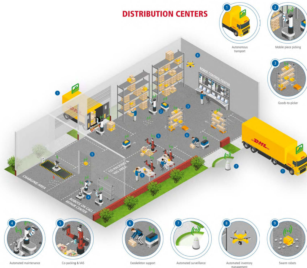
Figure 1.3: Distribution center concept showcasing various automated vehicles [7]
