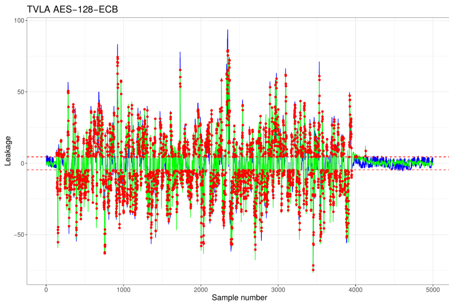
Figure 4.1: TVLA of AES-128-ECB using 2500 traces. One line is given for each run, the red points indicate leakage which was found in both runs.
