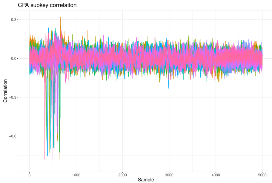
Figure 4.3: The correlation of the best keyguess at every point in time. Every line corresponds to one byte of the key.
