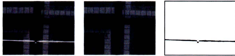
Figure 5.5: An image with projected laser beam is subtracted with an image without. [Kah04]
