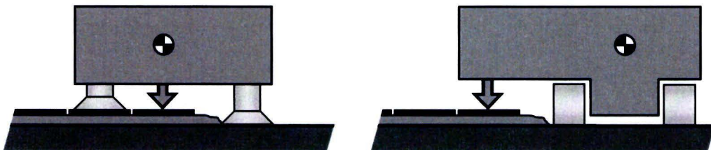
Figure 3.4: A walking robot with central placement versus a riding motion with eccentric placement.
