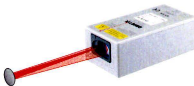
Figure 5.12: Dimetix FLS-C10 laser distance sensor [Dim].
