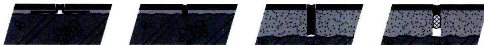
Figure 2.5: Various types of expansion joints: An embedded expansion profile or a joint sealant, either applied in thick-bed mortar or thin-set adhesive.
