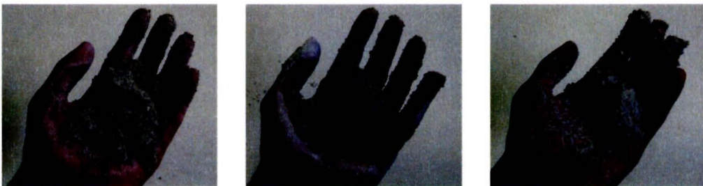
Figure A.9: Hand test to evaluate moisture level of mortar.
