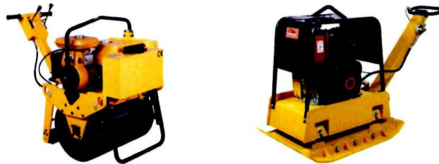
Figure 4.5: Vibratory equipment used for sand compaction.
