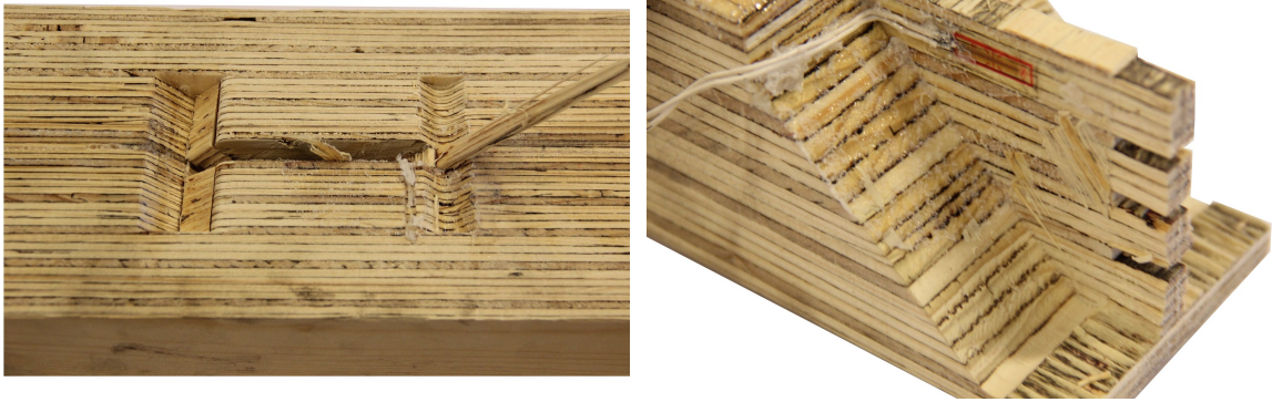
Figure 6.9: Failed connection test 1
