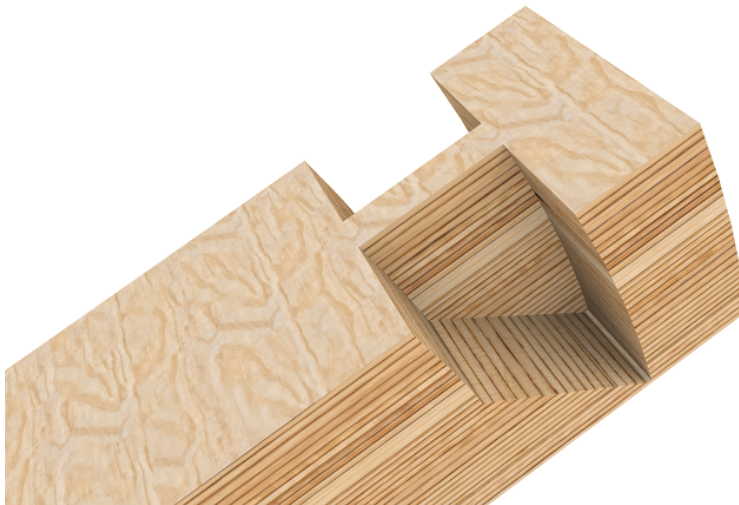
Figure 4.8: Diagonal with optimal dimensions in BauBuche Q
