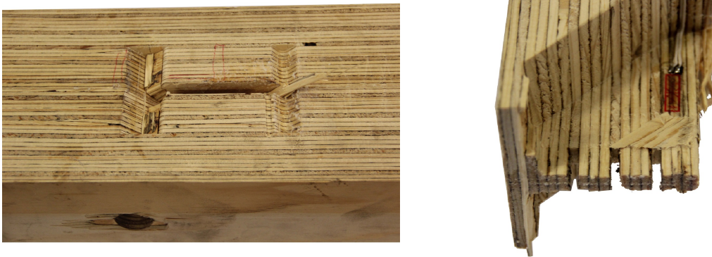
Figure 6.10: Failed connection test 2
