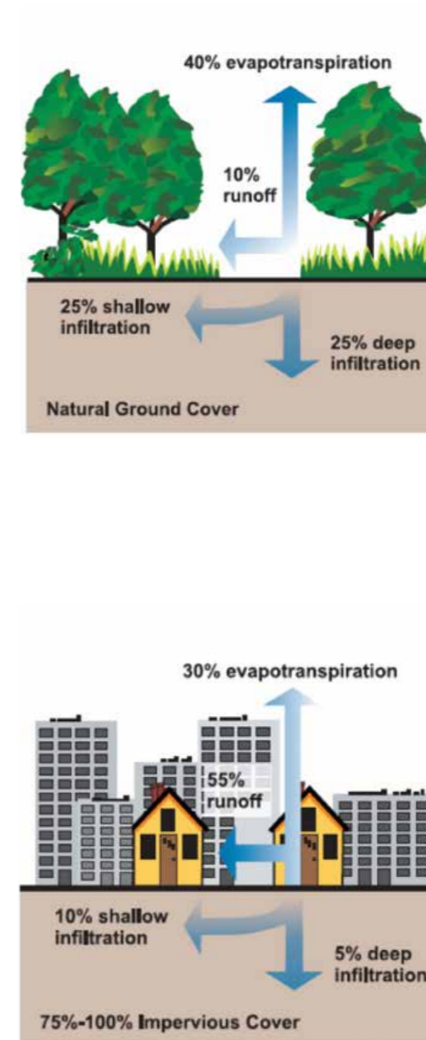
Figure 2.03 Rainwater processing in natural and urban environments (STOWA, n.d.)
