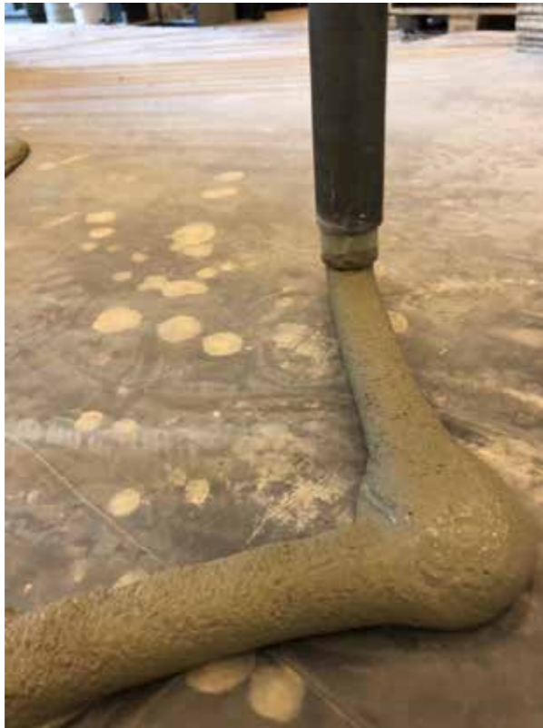
Figure 2.15 Printing without a nozzle
