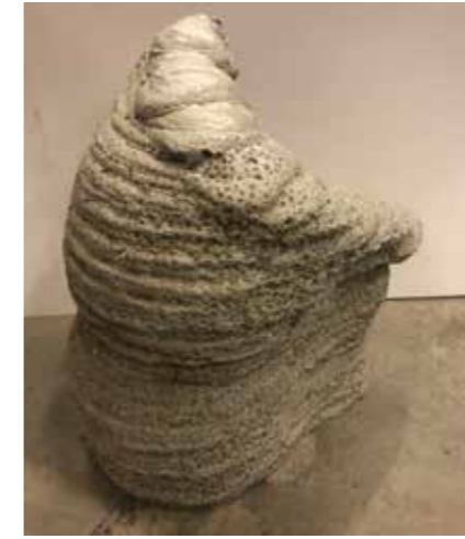
Figure 2.29 3D model printed using glass beads as support material
