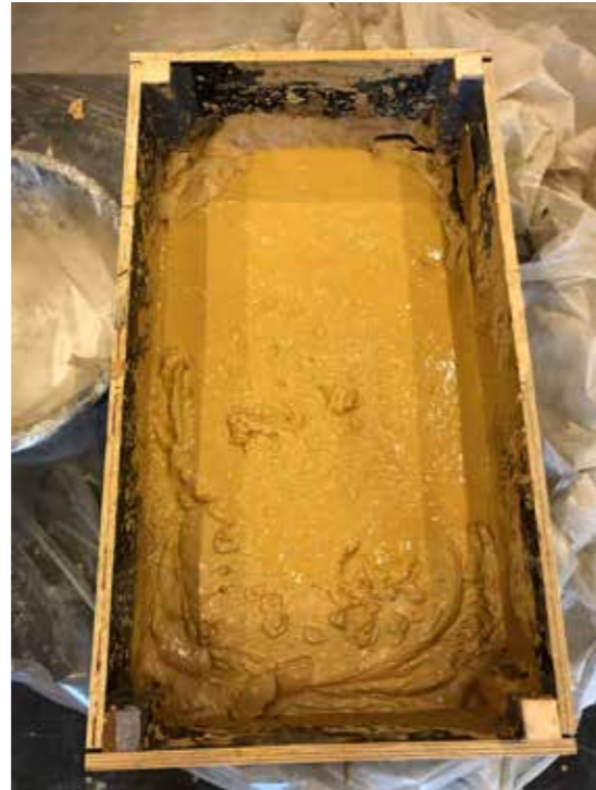
Figure 2.20 A more sturdy plywood box replaced the plastic box
