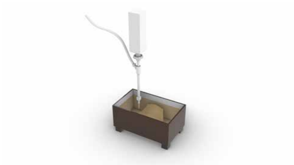
Figure 2.21 Schematic visualization of 3d injection printing inside a box with clay
