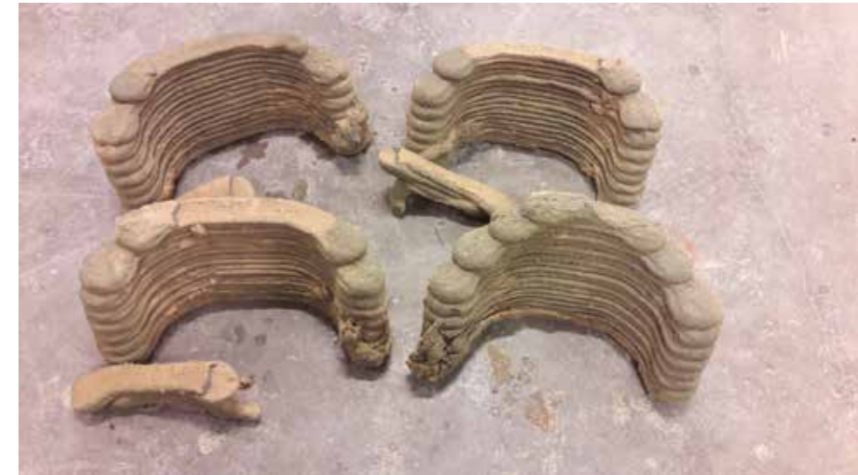
Figure 2.31 Slightly double-curved object printed using CLIP
