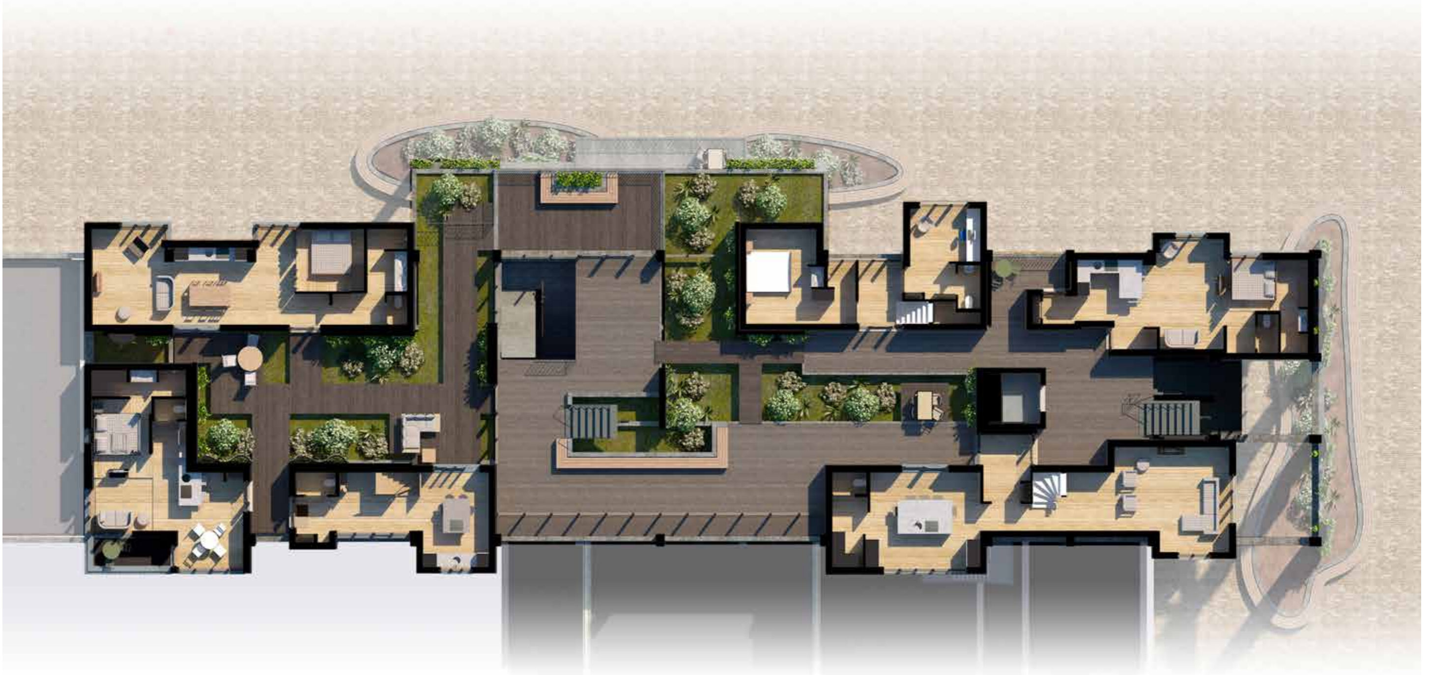
Drawing 5.35 Plan showing the new layout of the roof, featuring a green communal area with adjacent dwellings and green facades
