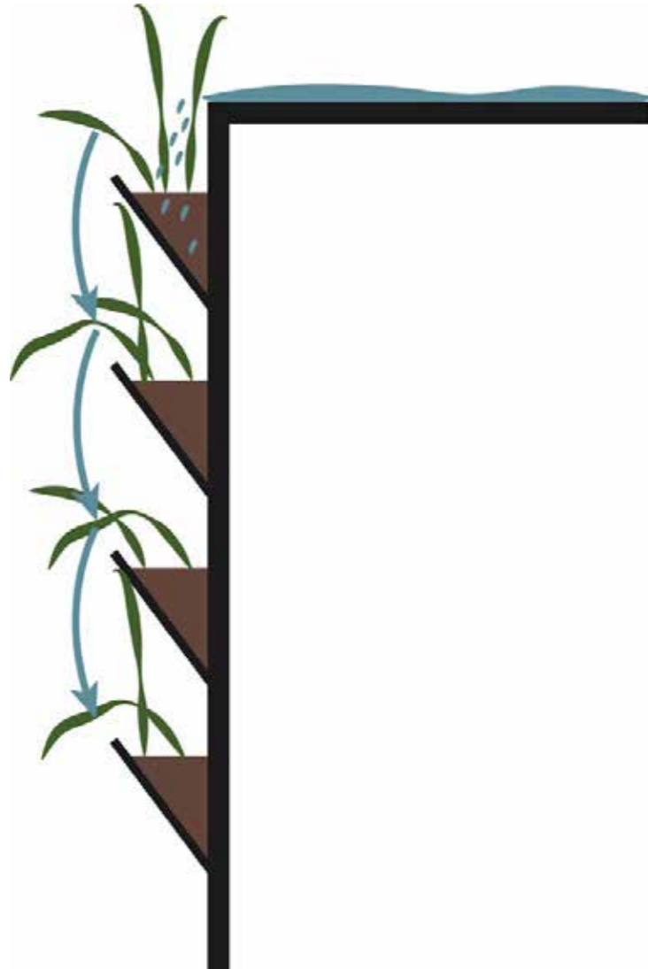
Drawing 5.9 Scheme explaining the concept of the green facades storing and draining rainwater from the rooftops
