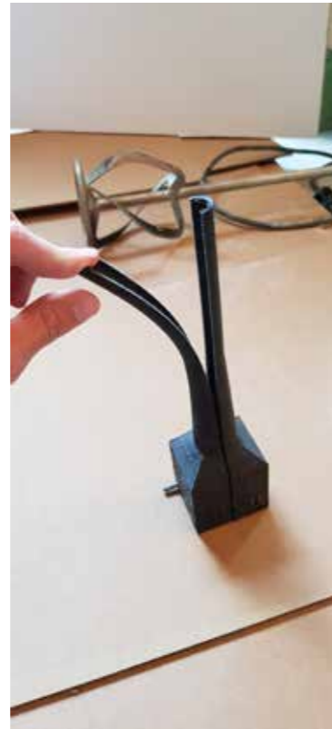
Figure 2.16 Nozzle made of flexible TPU
