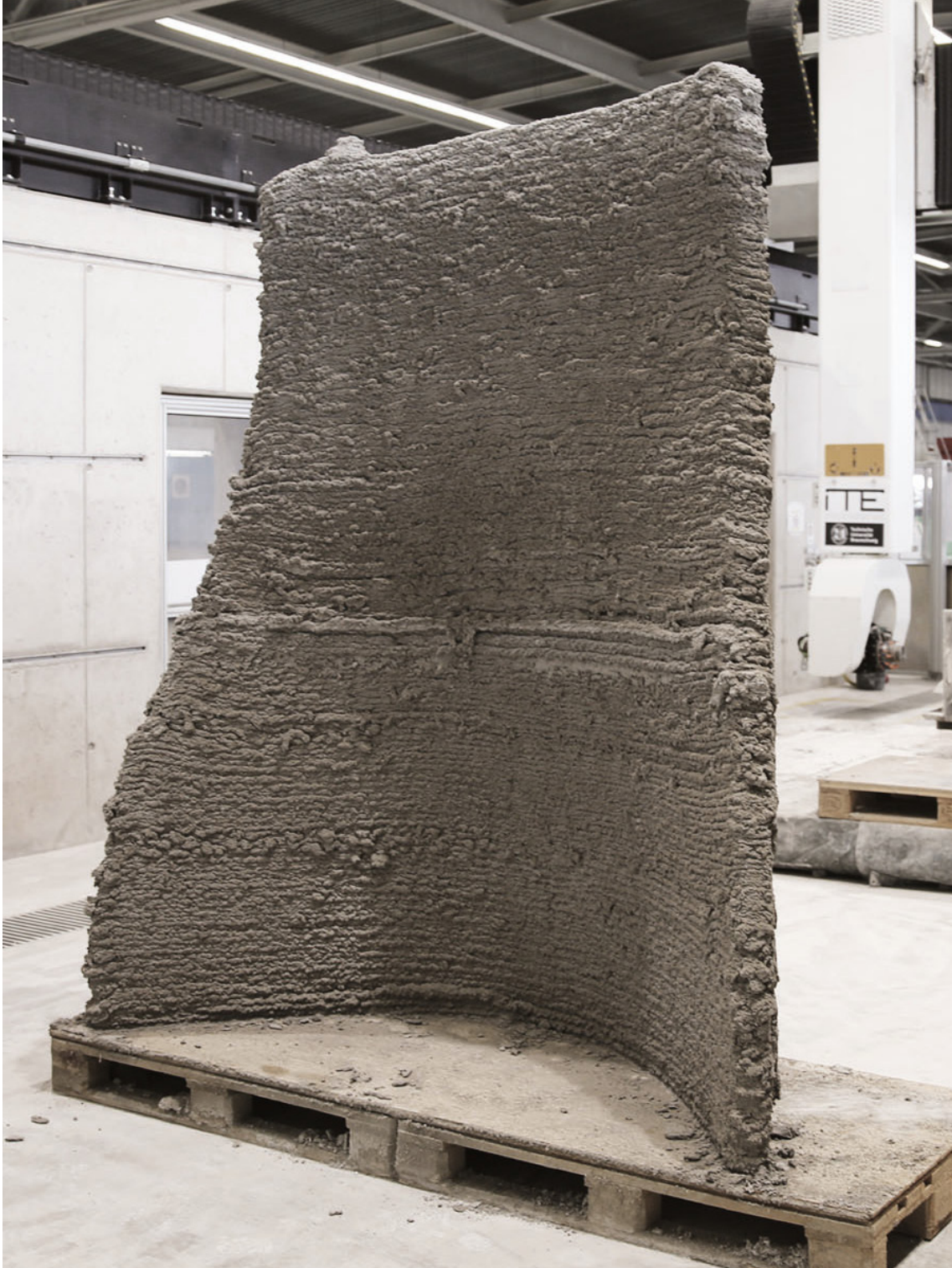
Fig 3.1: Double Curved 3D Concrete Spray Printed Wall [38]
