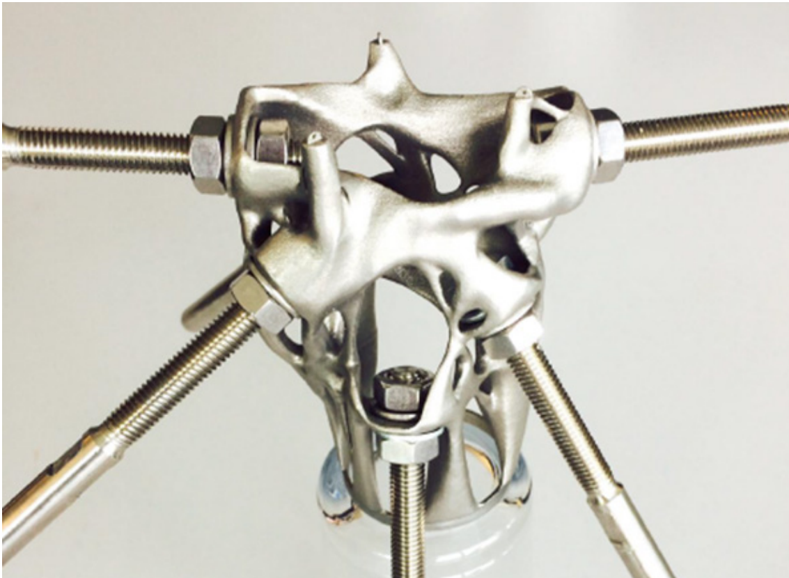
Fig 4.5: Arup's stainless steel AM node with connecting threaded swaged ends to the cables. [55]
