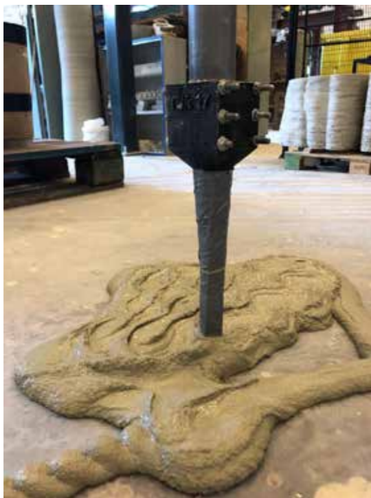
Figure 2.17 Reinforced nozzle with steel rod taped to the TPU
