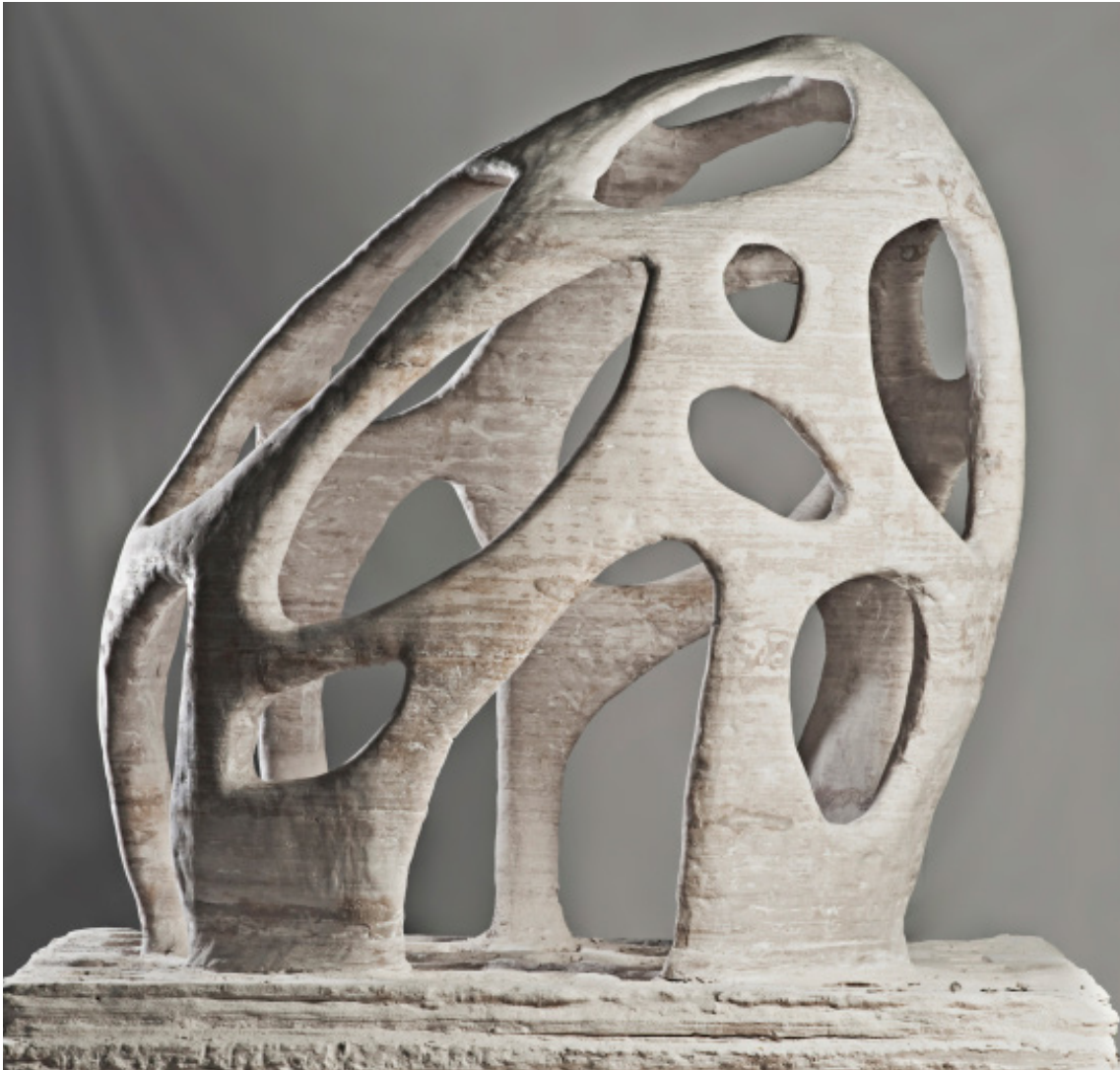
Fig 3.2: Radiolaria Pavilion printed by Dini's D-Shape Printer [42]
