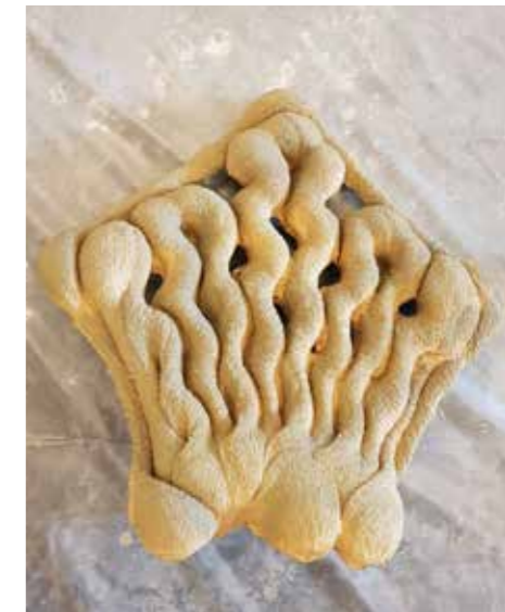
Figure 2.28 Flat pentagon printed on a dry printbed
