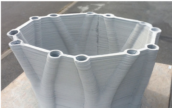
Fig 4.9: 3DCP pushes the limits of construction
