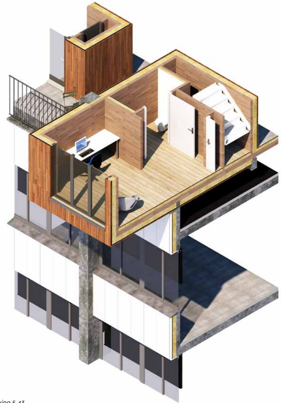
Drawing 5.43 Axonometric section of the existing facade and dwellings resting on it
