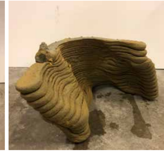
Figure 2.30 Similar 3D model print using clay as support material
