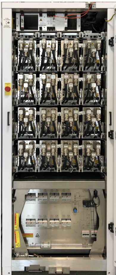
Figure 1.1: A power cabinet filled with power amplifiers, the subject of this project
