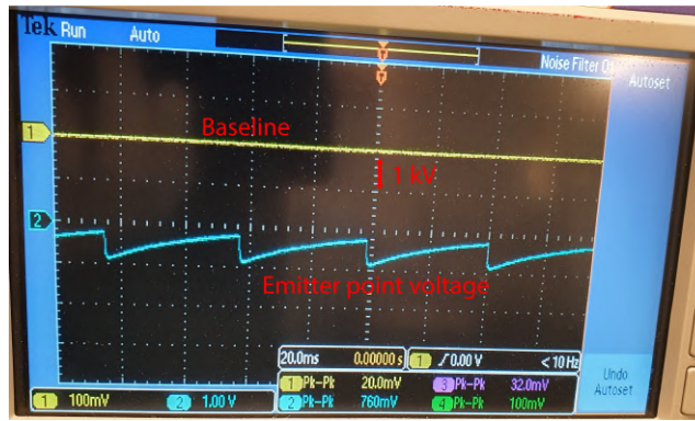
Figure 79: The frequency and voltage of a negative emitter point.
