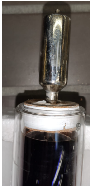
Figure K.2: Solution to prevent that the condenser slides down into the evacuated tube: teflon tape around cork.
