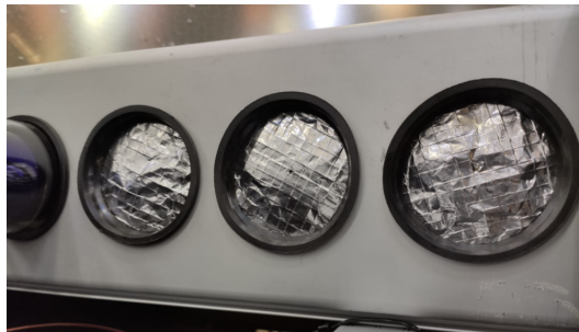
Figure 3.4: Insulation of the empty manifold holes
