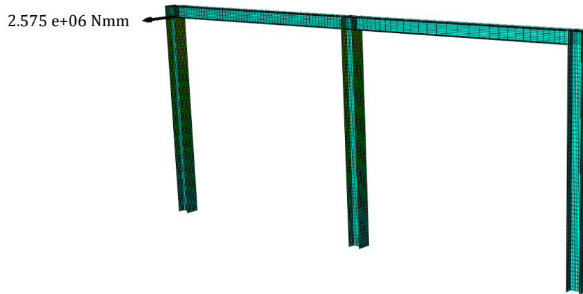
Figure 53: Resultant of section-moment EI|\eta_{cr}''|_{max} for the eigenmode of Figure 52, plotted on the undeformed state
