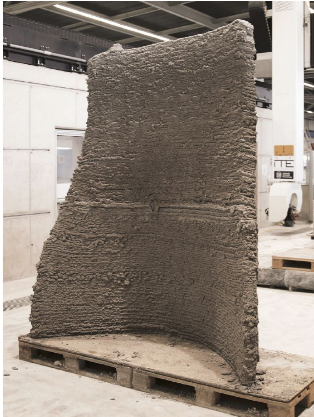
Fig 3.1: Double Curved 3D Concrete Spray Printed Wall [38]
