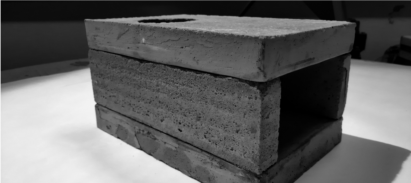
A concrete model with a rammed concrete wall and the circular skylights.
