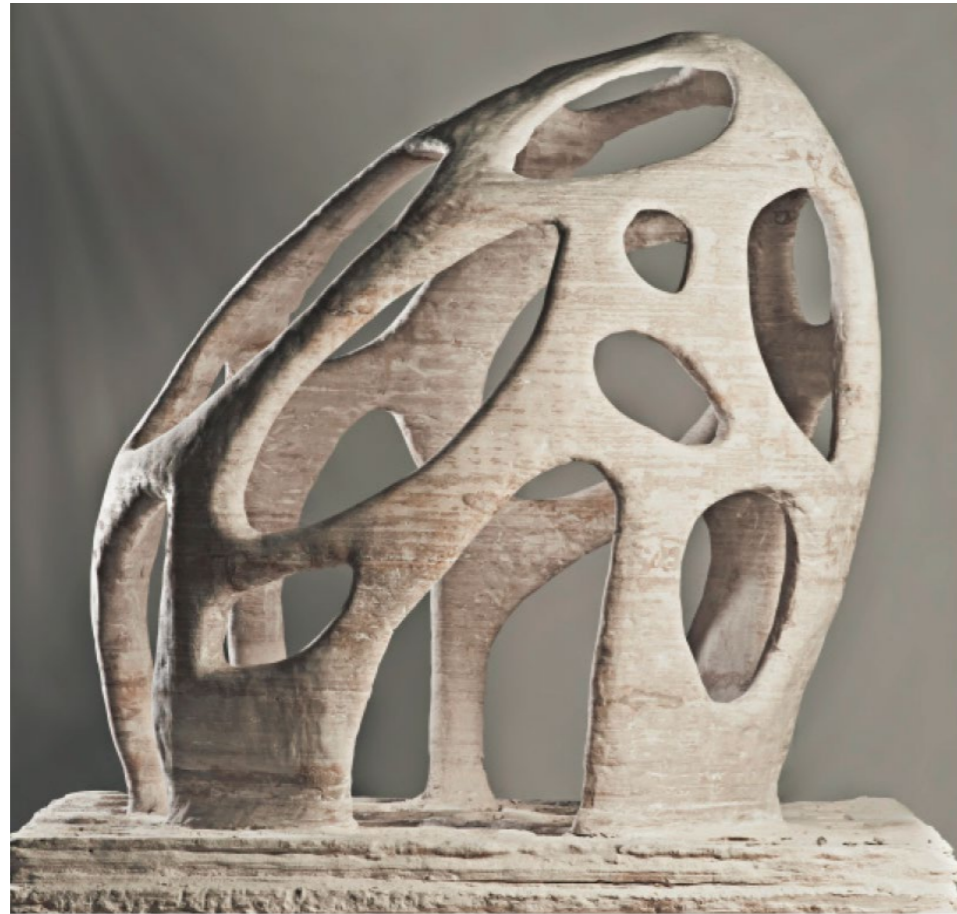
Fig 3.2: Radiolaria Pavilion printed by Dini's D-Shape Printer [42]
