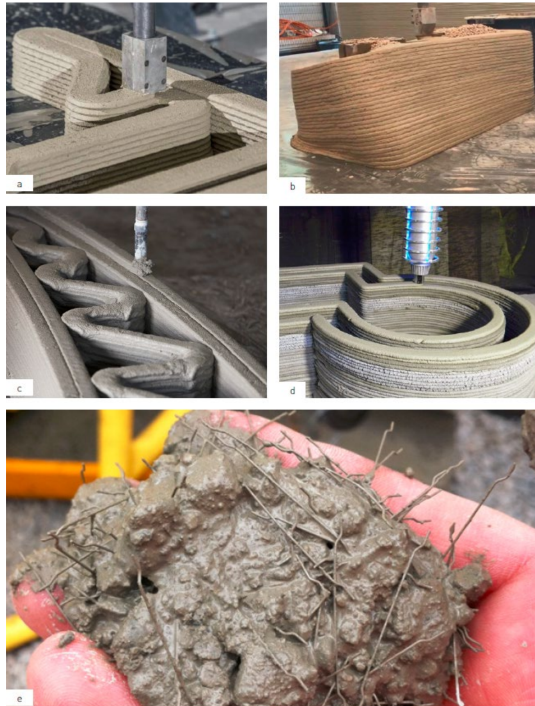
Fig 4.3: a: Consistent extrusion, b: Buckling due to inappropriate buildability, c: Support structure to improve buildability, d: Bonding between layers, e: Addition of fibers
