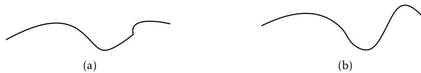
Figure 1.5: (a) A continuous curve containing a sharp bend, making it C^0 -continuous. (b) A (smooth) continuous curve with a continuous derivative, making it C^1 -continuous.
