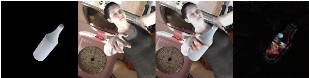
Figure 7.12: From left to right: object mask, source image, generated image, SSIM difference map. The hand parts that should be shadowed by the object are not.
