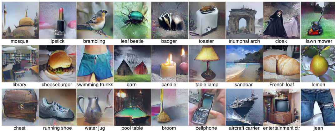
FIGURE 2.4: Input samples that maximize activation of output neurons in the CaffeNet deep neural network, which has learned to classify different types of ImageNet images [75].
