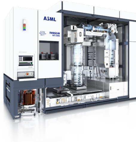
Figure 1.1: The latest DUV lithography system NXT:2000i as seen on the website of ASML
