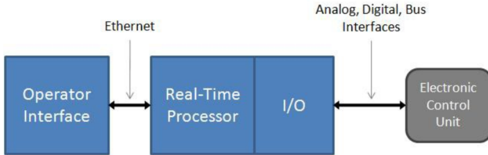
Figure 2.3: Components of a HIL simulation[3]
