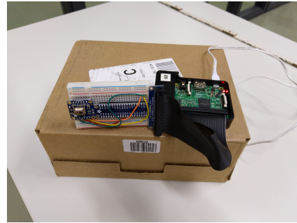
Figure 5.10: Wireless sensor node consisting of a Raspberry Pi 3 model B and the AMG8833 breakout board.
