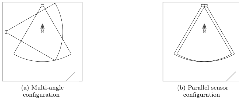
Figure 4.2: Examples of sensor configurations for multi-sensor posture recognition
