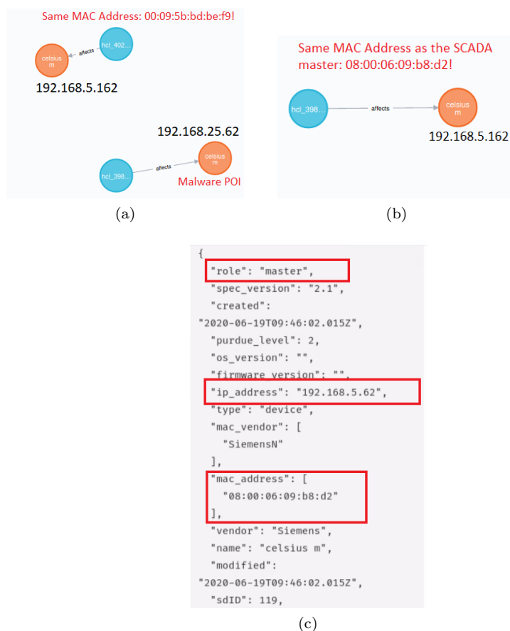
Figure 6.8: Malware POI Impersonating a SCADA Master Device
