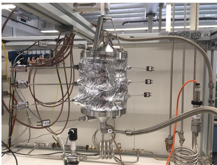
Figure A.3: Picture taken from the reactor after wrapping exhaust wrap around the steel layer. The exhaust wrap is held in place by means of metallic tape
