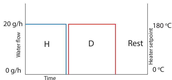
Figure 2.11: A normal hydration to dehydration cycle over time. The blue line represents the water flow over time, while the red line represents the heater temperature. In the area marked with H, hydration takes place. Afterwards, dehydration is almost immediately started (D). After the material is dried, the reactor is left at rest in order to cool down to ambient temperature over time. No flow is active during the resting period, and the reactor is closed using valves. This prevents water vapor from the surroundings to enter the setup.
