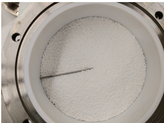
Figure H.1: Height of the particle bed before the first run
