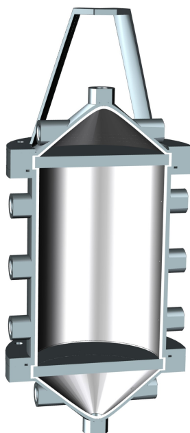
Figure 2.3: The inside of an assembled reactor. Air flows in from the top, through the glass filter and the packed bed (not shown on this picture). The horizontal extractions are used for placing thermocouples at the inside of the reactor.
