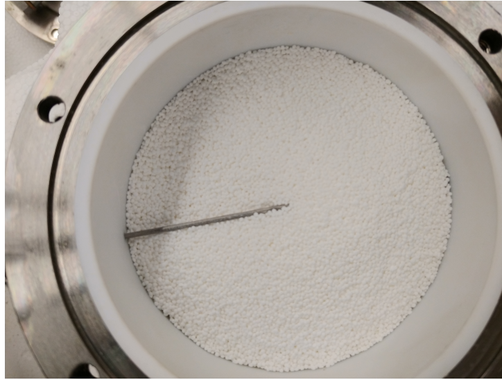
Figure 5.2: Height of the particle bed before the first run
