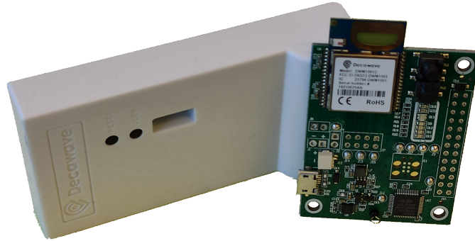
Figure 2.3: Decawave’s DWM1001 Development Board. Hardware used for anchors and tags of both UWB-based localization systems utilized in the experiments.
