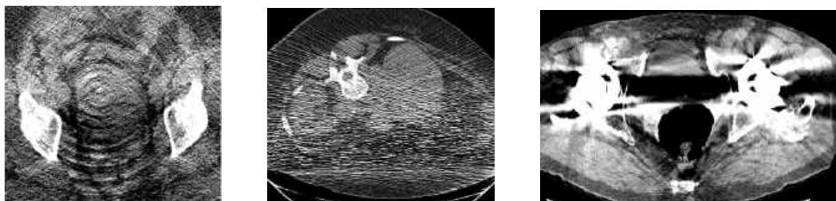
Figure 1.1: Examples of CT image artifacts: (a) Ring Artifact (b) Poisson Noise (c) Beam Hardening and Scatter Artifacts (Source: CT artifacts: Causes and reduction techniques)
