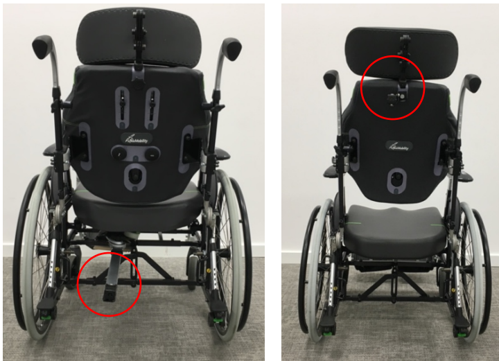
Figure 7 – Left: modification based on largest cluster from intuitive method (first choice intuitive wheelchair). Right: modification based on smaller cluster from intuitive method (second choice intuitive wheelchair).
