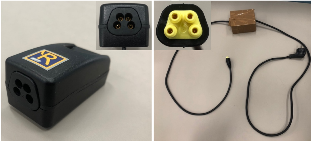
Figure 2 - Left: R-net female charging port that was fitted on the wheelchairs. The yellow logo was taped off in the experiment. Right: prototype charger.
