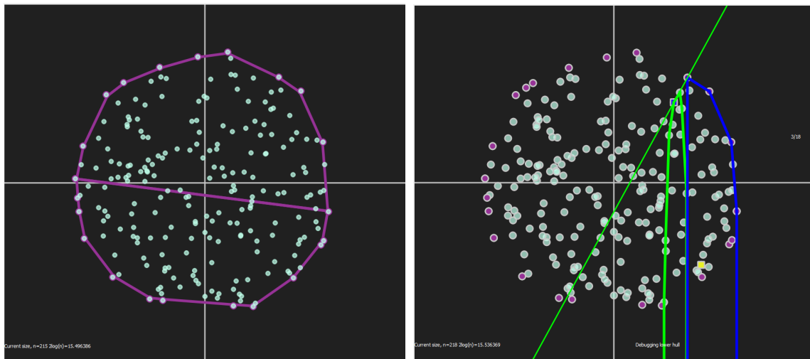
Figure 6.4: An example of how the debugger works. On the left we see a complete convex hull and on the right we see one of the steps of updating the upper hull after an insertion. The lower hull can be debugged in the same way. The steps to find the bridge are also able to be inspected. It displays some information about the current case, like what the average size of the number of steps should be: 2 \log n for the current n . A similar debugger was made for envelopes.
