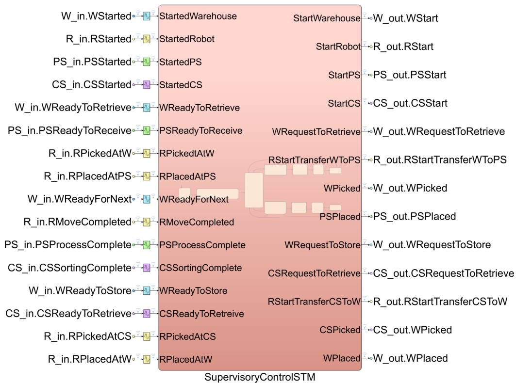
Figure 4.2: Inside the Supervisory Control subsystem in Simulink.
