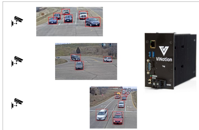
Figure 1.2: Multi-camera single platform solution
