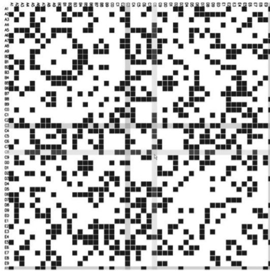
Figure 3.4: An undirected graph(50 nodes and 400 edges) in matrix representation.
