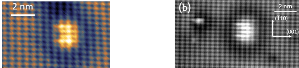
(a) Second layer Si donor in AlAs as observed in our measurements. (-2.7V, 30pA) (b) Si donor in GaAs as observed by Feenstra et al. [57]. (-2.2V)
