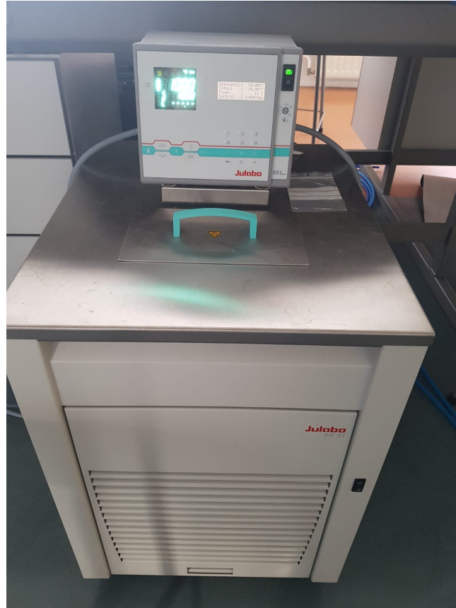
FIGURE 4.10: Circulation thermostat that is used to control the temperature of the gas inflow of the experimental setup
