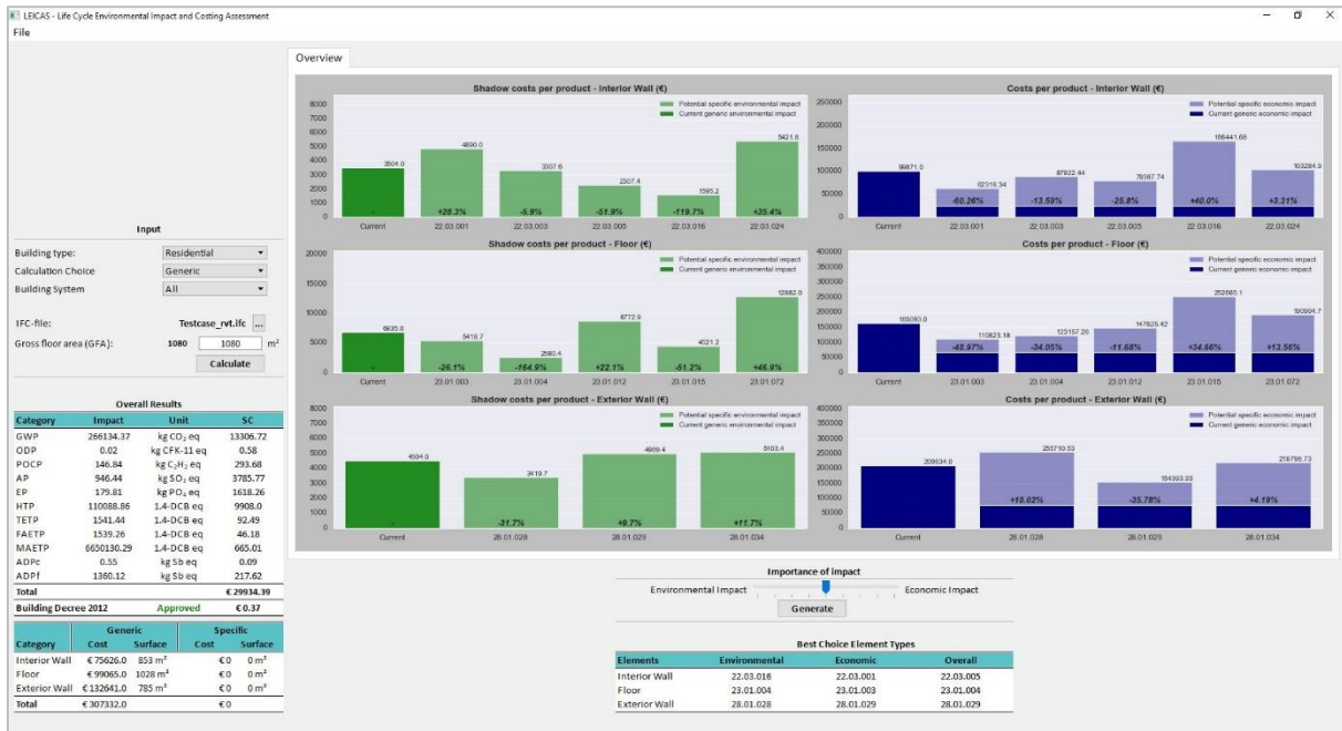
Figure 27 - Snippet with results of the generic scenario based on building system "All"
