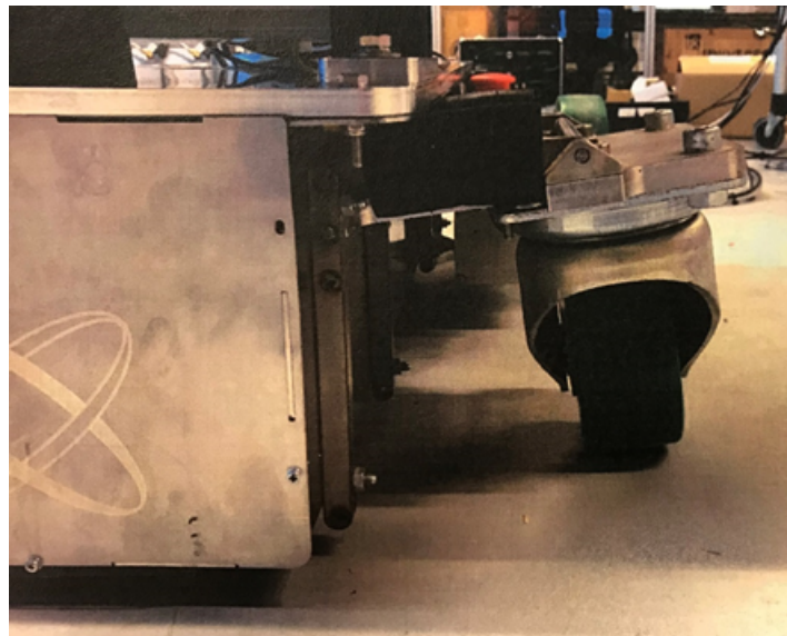
Figure 1.4: Sagging of the AGV's suspension
