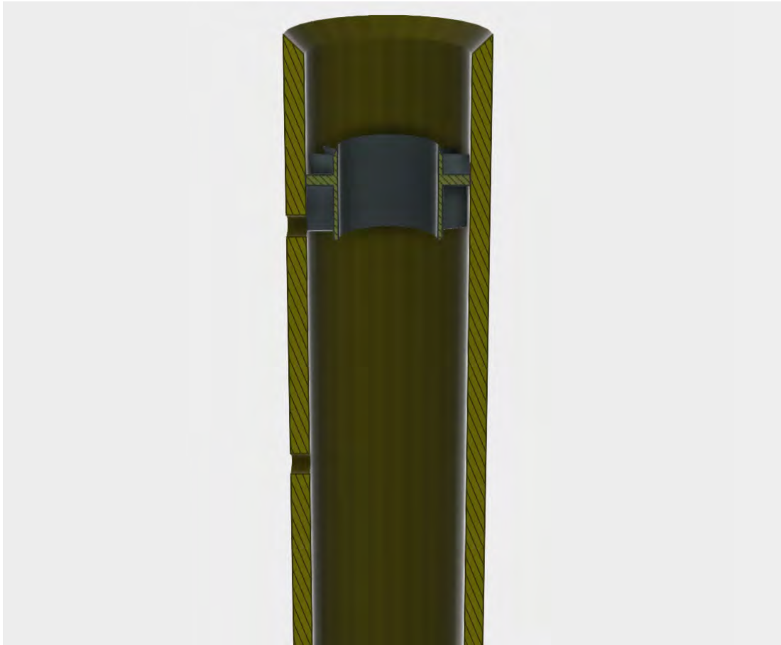
Figure E.2: Close up of the swirler inside the burner.
