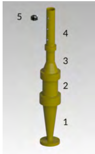
Figure 5.1: Graphical description of the Low Swirl Burner
