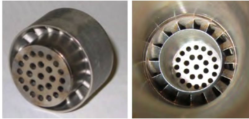
Figure 4.3: Low Swirl Injector, back view (left) and front view (right). From: [5]
