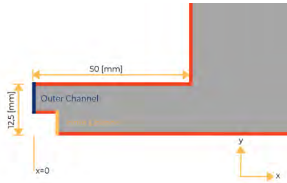
Figure 5.4: Sketch of the premixing zone for LSB TU/e
