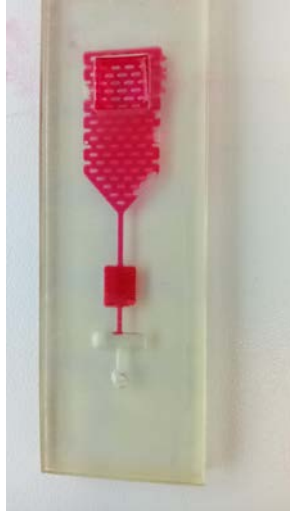
Figure 3.5: UV cured binding of cover-plate with the device
