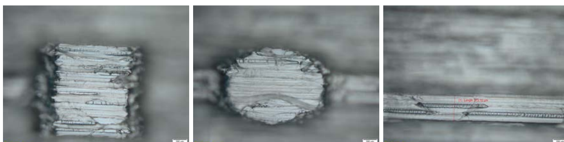
(a) chamber 1 (b) chamber 2 (c) channel 1 Figure B.12: Prints with Matte print setting printed in vertical orientation
