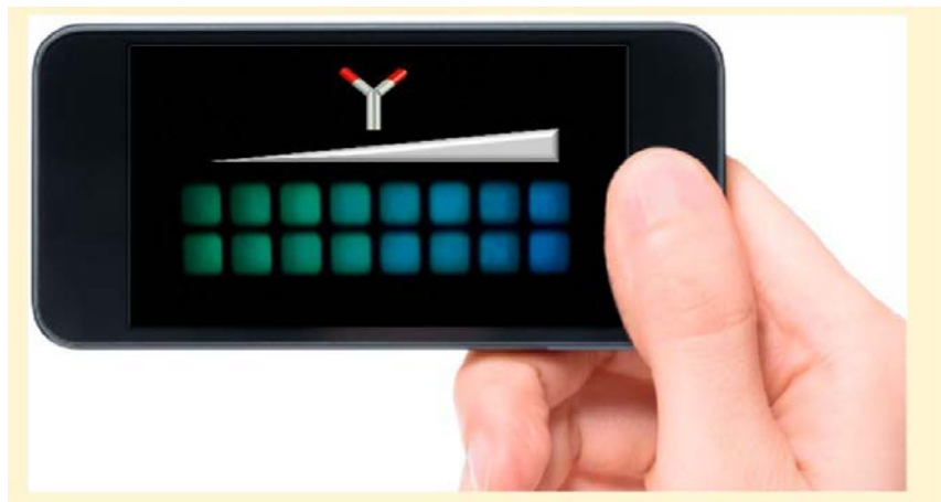
Figure A.3: Shift in color due to the interruption of BRET partners with binding of antibodies measured with a smartphone camera
