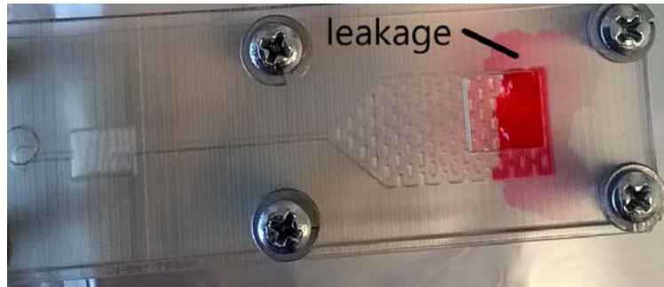
(a) leakage in bolted assembly
