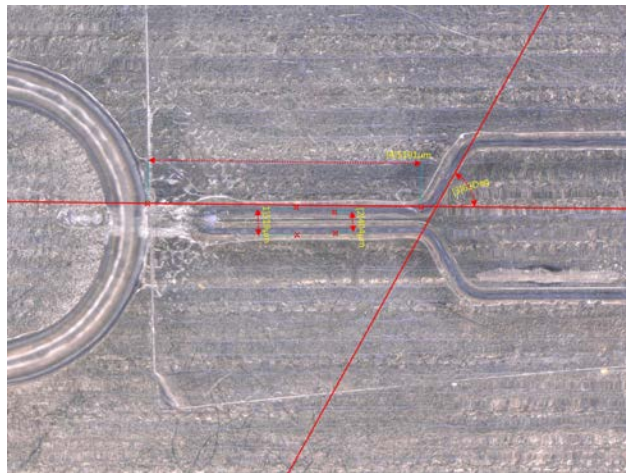
(b) 60° expansion with channel width measurements
