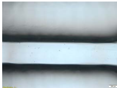
(d) Microchannel 4 printed with Glossy High Speed setting
