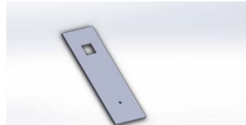
(d) Cover-plate bonded with double-sided tape
