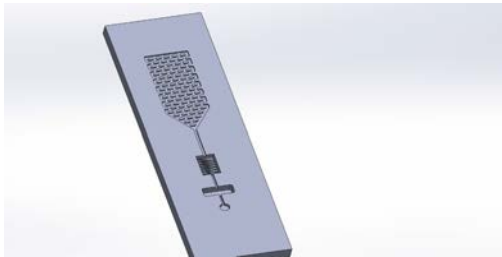
(c) Microfluidic device bonded with double-sided tape
