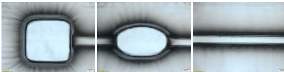
(a) chamber 1 (b) chamber 2 (c) channel 1 Figure B.9: Prints in Glossy print setting printed in horizontal orientation
