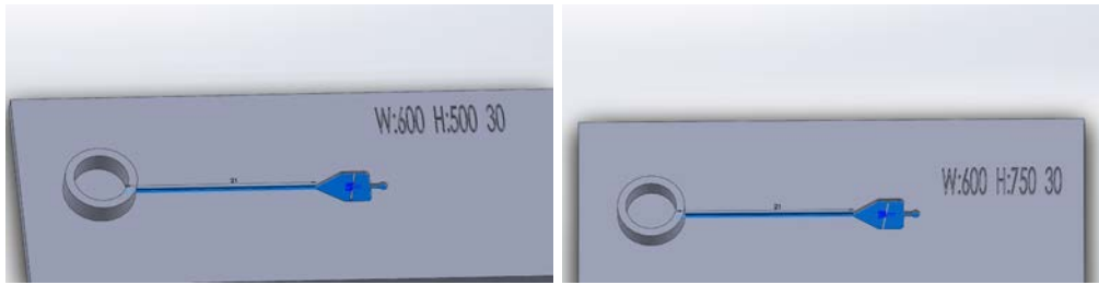
(a) Microchannel with depth 500\mu m and width 600\mu m (b) Microchannel with depth 750\mu m and width 600\mu m
