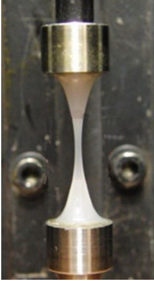
Figure 2.2: Polymer sample between two pistons in a filament stretching extensional rheometer (Image reproduced from [26]).
