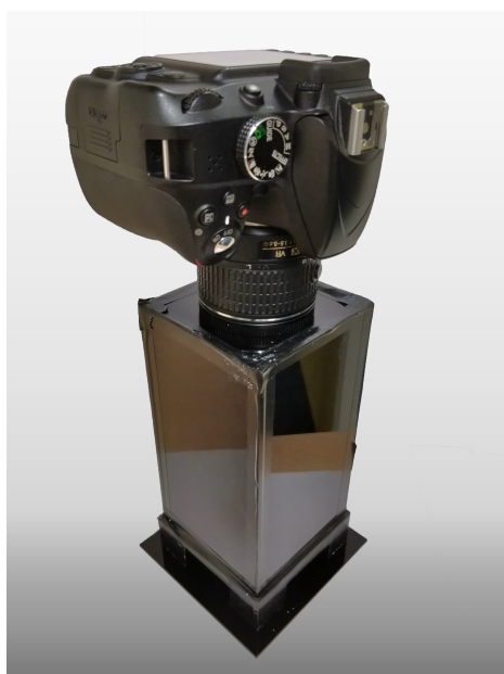
Figure 3.6: Luminescence detection set-up. Nikon D3300 digital slr camera on a black box containing the POCT chip. Dimensions hxwxd: 200x90x90 [mm].
