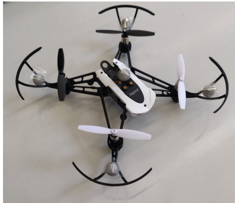
Figure 5.2: Configuration of the Optitrack balls: four in the corners and one in the center.
