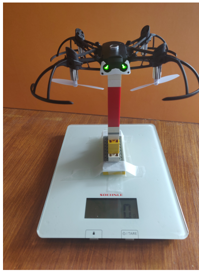
Figure 4.7: Setup of the thrust experiment: the drone is mounted upside down to a scale.
